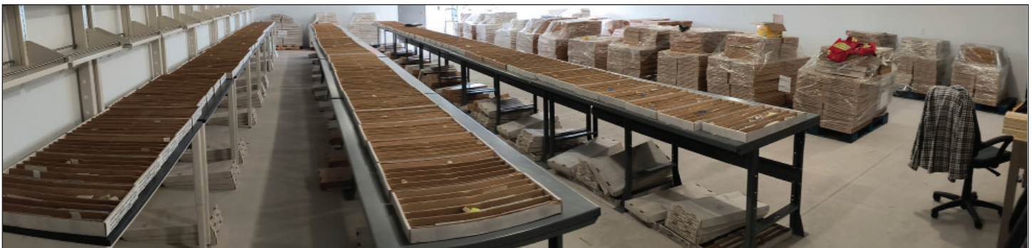
Drill core staged for sampling in the Mineral Storage Building.
