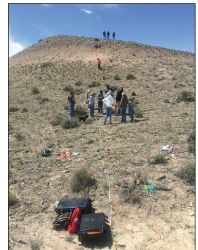
Characterization Program staff and University of Montana Western students testing geophysical equipment for use in locating buried valley aquifers.
