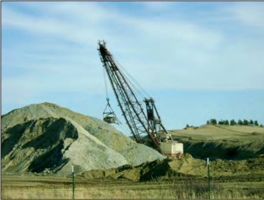
A dragline removes overburden and exposes the coal seam at Western Energy's Rosebud Mine near Colstrip, MT.
