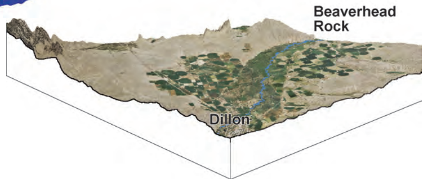
Detailed hydrogeologic data and land features are represented in a 3-D numerical simulation of the GWIP study area near Dillon. The model was used as a tool to evaluate stresses such as changing rates of groundwater withdrawal on surface water.
