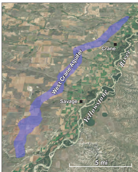
GWIP hydrogeologists, through drilling, identified the extent of the West Crane buried alluvial aquifer. The aquifer is capable of well yields up to 1,500 gpm.
