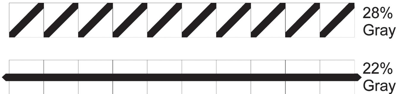
Figure 19. Two rows of vector-based point symbols centered in square grid cells. Symbols in the second row have been rotated  $45^\circ$  clockwise around the center of the grid cells. Overlap of the black point symbols in the second row results in a decrease in overall darkness between rows from 28% gray to 22% gray, a relative change of more than 20%.
