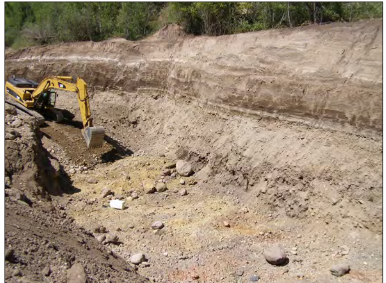
Placer exploration near Garnet. Note placer drift timbers from the previous century along bottom of the gravel.
