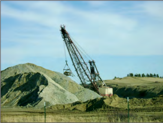
A dragline removes overburden and exposes the coal seam at Western Energy's Rosebud Mine near Colstrip, MT.
