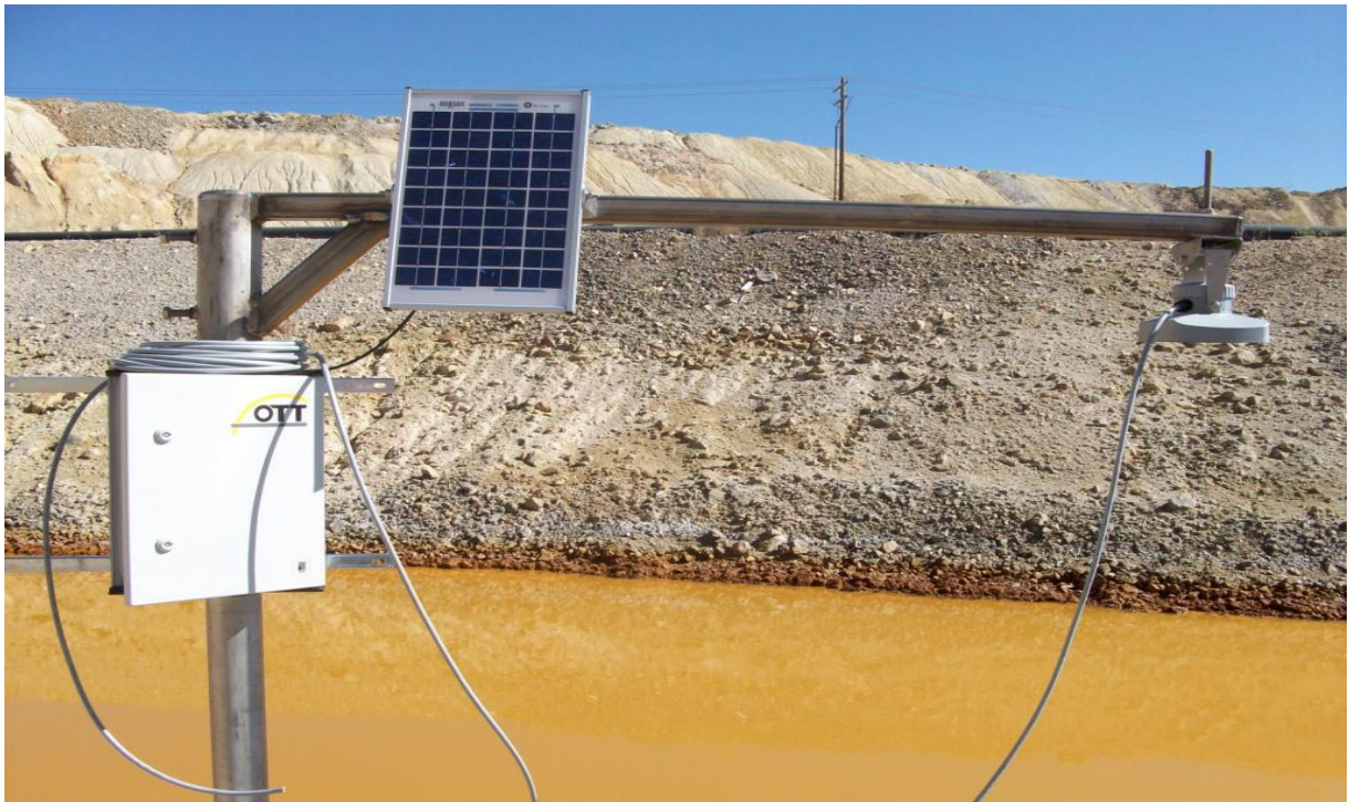
Figure 2-47. Radar system installation at the Horseshoe Bend weir monitoring station.
