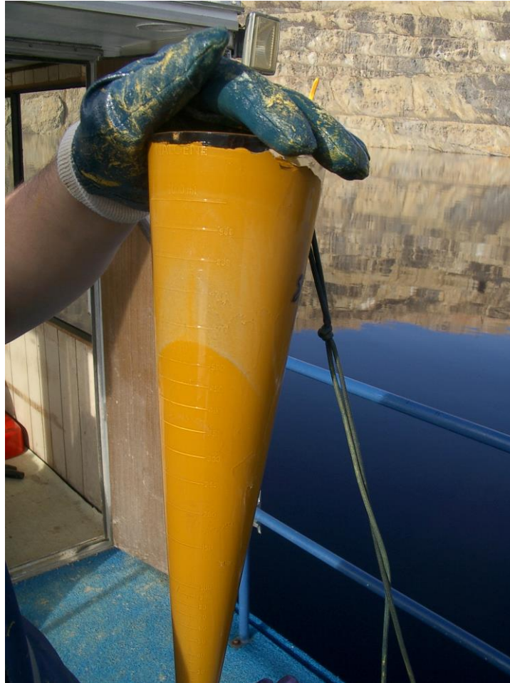
Figure 2-55. Accumulation of secondary iron precipitates in a sediment trap deployed in the Berkeley Pit for 150 days.
