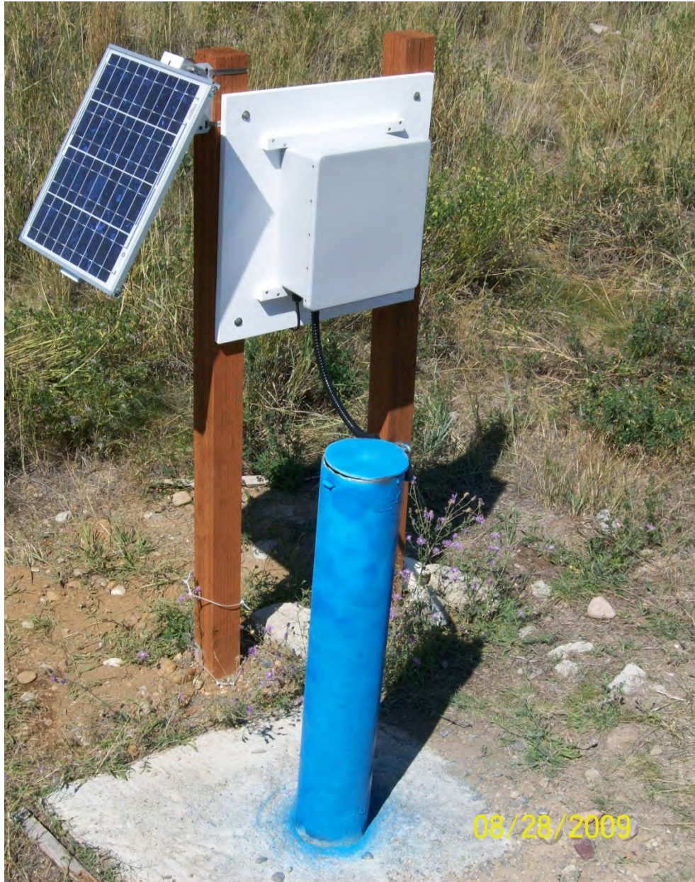
Figure 4.2-7. Telemetry system installed at well MW-213.
