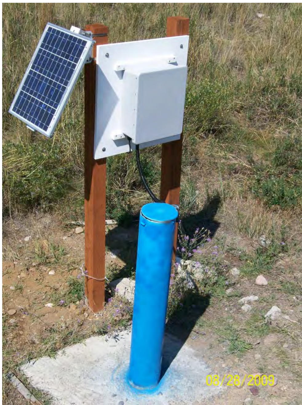
Figure 4.2-7. Telemetry system installed at well MW-213.
