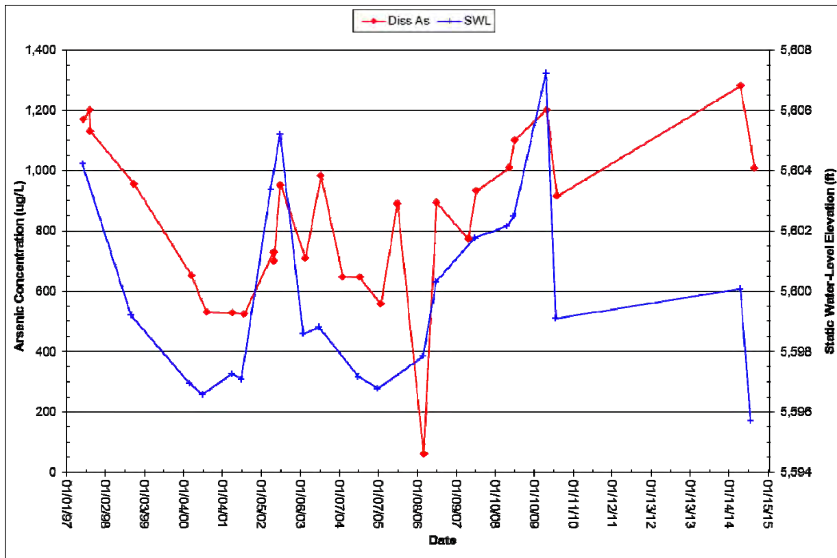
Figure 4.2-4. Well MW-245S, located on Smelter Hill: arsenic concentrations and static water-level elevations over time.
