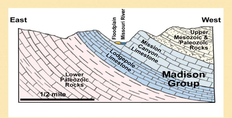
Geologic cross section showing the dipping beds that may have appeared to Lewis "to have tumbled or sunk."
