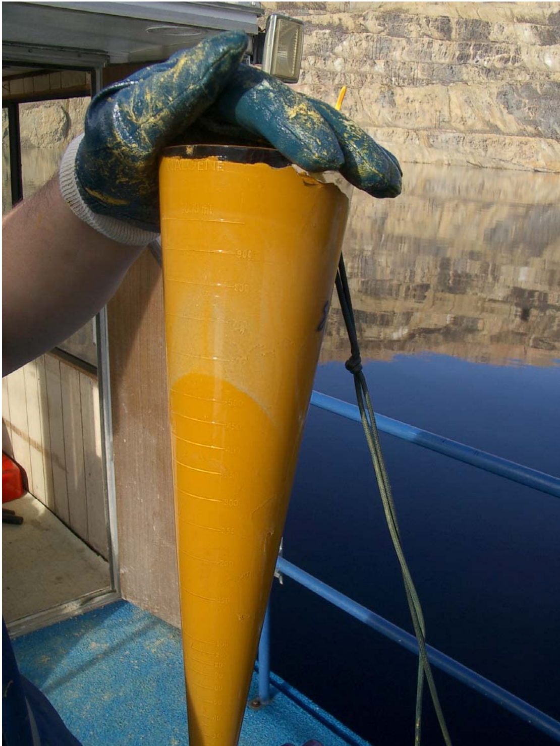
Figure 2-54. Accumulation of secondary iron precipitates in a sediment trap deployed in the Berkeley Pit for 150 days.
