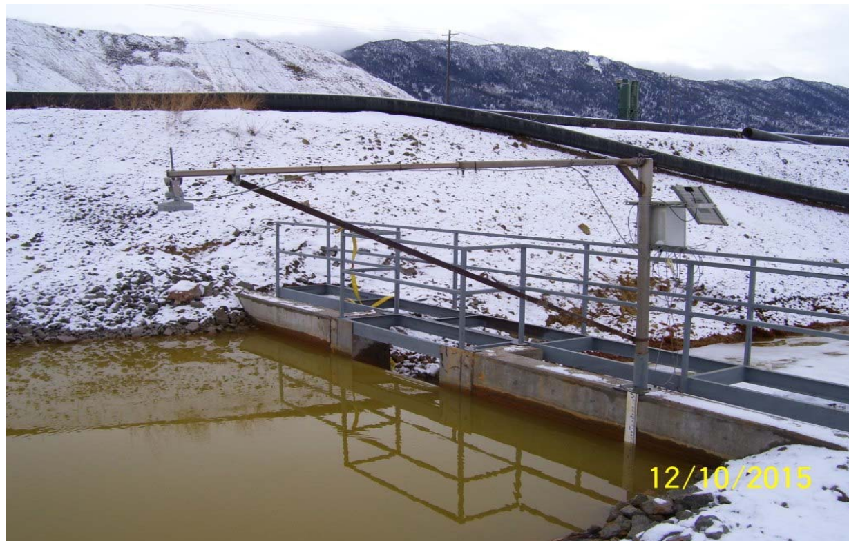
Figure 2-46. Radar system installation at the Horseshoe Bend weir monitoring station.
