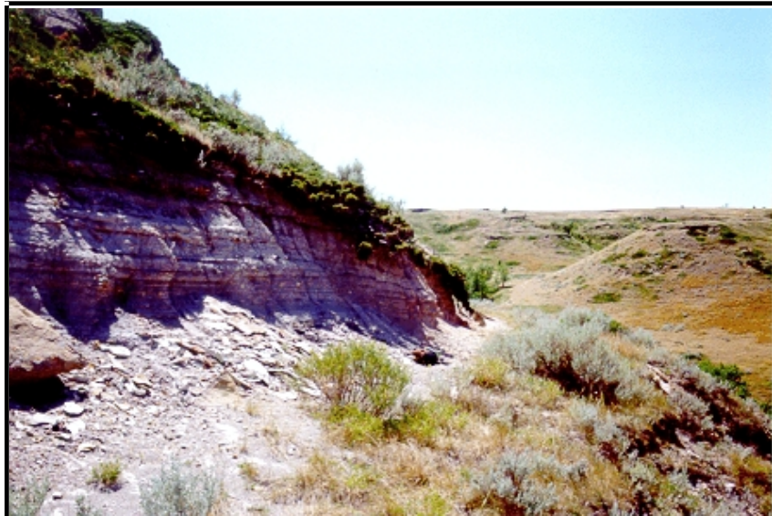
Bulldozer cut into hillside exploring a lignite seam. Sloughing from the cut bank has mostly covered the lignite bed. Soil sample SCH3A was collected from this cut.
