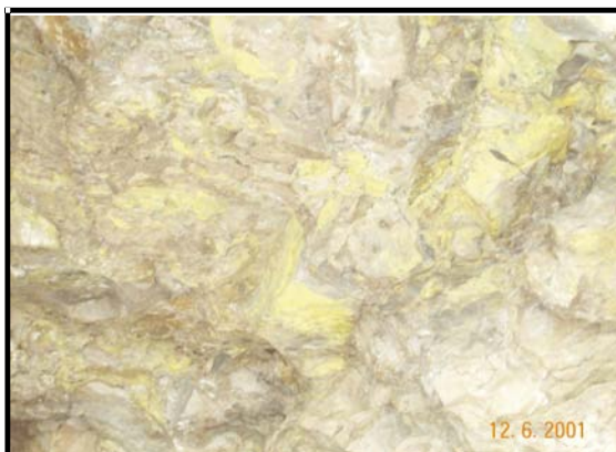
Visible uranium ore in roof of a shallow adit in Madison limestone of the Sandra Mine.
