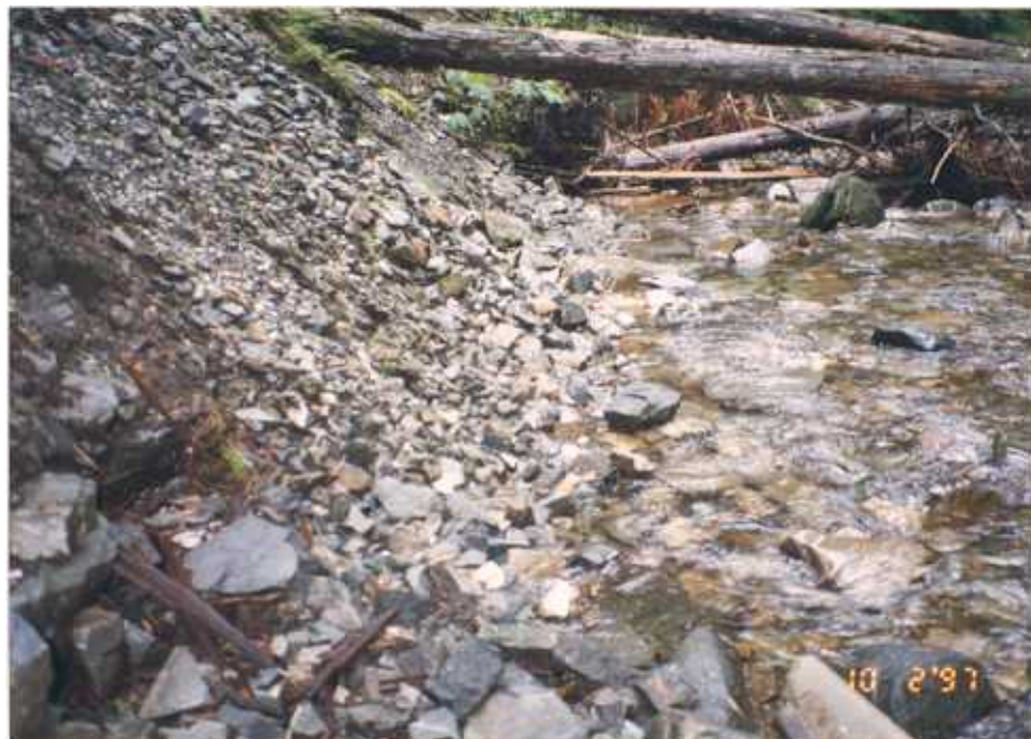
Figure 31b. The sparsely vegetated waste dump was in direct contact with Goat Creek. The large size of the fragments that compose the dump inhibits erosion of the waste.
