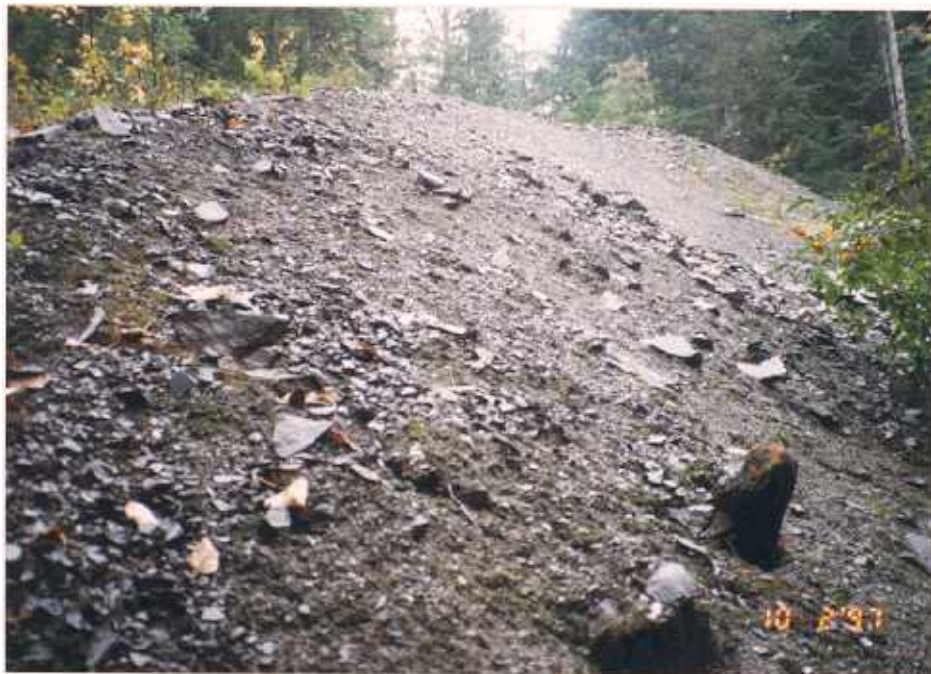
Figure 29b. The waste dump had been eroded by runoff, and a small seep flowed from the base of the dump.
