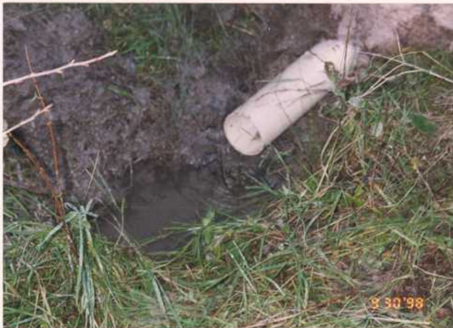
Figure 12b. The small rate flow at Rock Lake was measured as it flowed from the adit and was captured by a short piece of PVC pipe.
