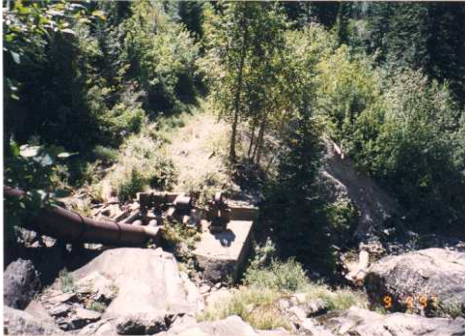
Figure 7a. As viewed from above, the Heidelberg mine consisted of a discharging adit, remnant mining equipment, and a waste dump that was in contact with Rock Creek.
