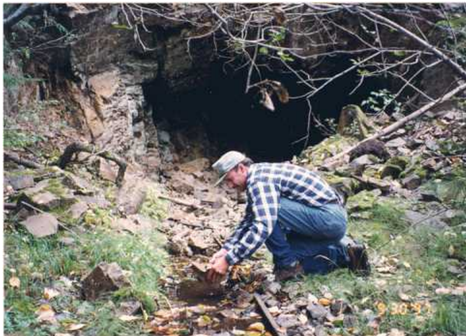
Figure 32b. The adit discharge from the open adit at the Snowstorm was sampled in September 30, 1997. The total flow was estimated at five gpm.
