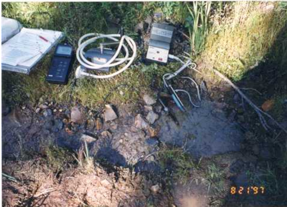
Figure 5b. Sample VVRS10M at the Vermilion River adit was taken from a small pool of water formed by the five-gpm adit discharge. It was taken on the north side of the road.
