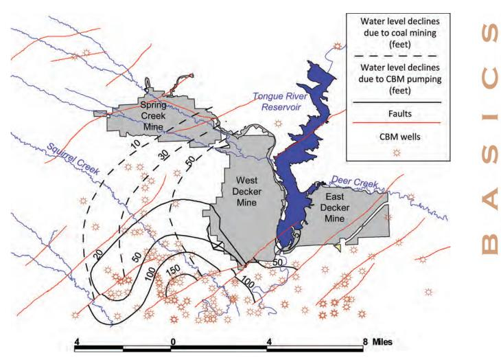
Figure 9. Water-level declines from mining of 10 feet extend farther than 5 miles beyond the West Decker coal mine after 25 years of mining. Aquifer drawdown from CBM production is approximately 20 feet at distances of 1 to 2 miles beyond the active CBM development area after 10 years of production.
