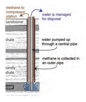
Figure 1. Coalbed methane is produced by completing a well in the target coal seam and pumping water from that coal. The stratigraphic column illustrated here is an example of typical Fort Union Formation geology.
