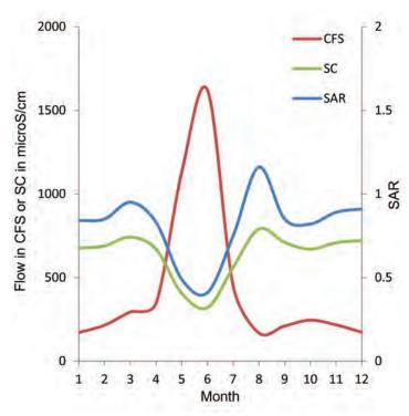
Figure 12. Average monthly flow rate, salinity (SC), and sodium adsorption ratio (SAR) for the Tongue River at the state line (U.S. Geological Survey, 2011).
