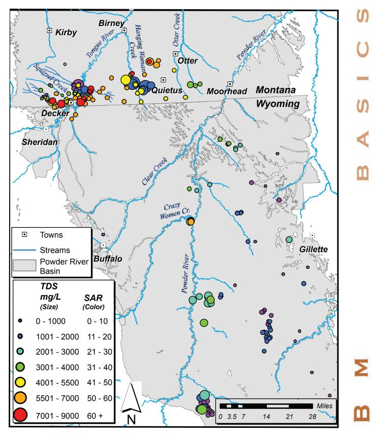
Figure 11. Sodium adsorption ratio (SAR) tends to increase with distance away from recharge. Mature coal aquifer water has TDS values between 1,500 and 2,500 mg/L, with sodium and bicarbonate being the dominant ions. Montana coal aquifer data from the Montana Bureau of Mines and Geology GWIC database. Wyoming coal aquifer data from Campbell and others (2008).
