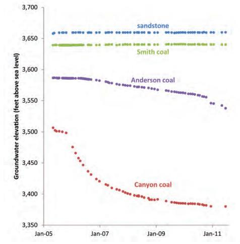
Figure 10. Drawdown in the Anderson and Canyon coals due to CBM production is not typically translated to the overlying coal and sandstone aquifers. GWIC ID numbers of the nested well set presented here are, top to bottom: 219617, 219138, 219139, and 219140.
