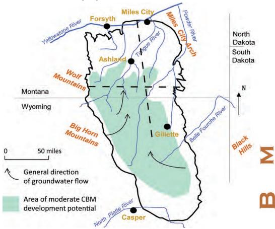
Figure 3. About one-third of the Powder River Basin is in Montana; however, less than 4 percent of the CBM resource is in Montana (Department of Energy, 2002; Van Voast and Thale, 2001). Dashed lines indicate locations of geologic cross sections shown in figure 5.
