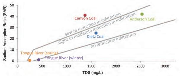
Figure 13. The effect of irrigation water on soil structure is dependent upon the TDS, the SAR, the soil type, and clay mineralogy (based on Hanson and others, 1999). Tongue River chemistry is reported from a station at the Wyoming/Montana state line maintained by the U.S. Geological Survey.
