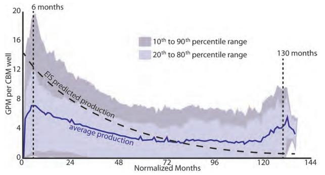
Figure 7. The average CBM well produces less water than the environmental impact statement (EIS) predicted for the first 6 years. Water production levels off in about 4 years at approximately 4 gpm. The range in production rates is shown by the shaded fields (data from the 2010 water year; Meredith and others, 2011).
