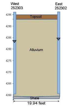
Figure 21. Well completion diagram for observation well 252303 and pumping well 252302. Water levels used for the diagram were measured on 8-25-09.
