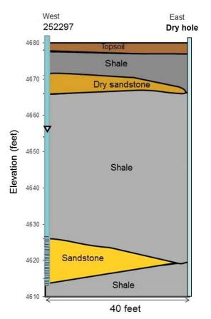
Figure 38. Well completion diagram for a well (252297) drilled into the Hell Creek aquifer.
