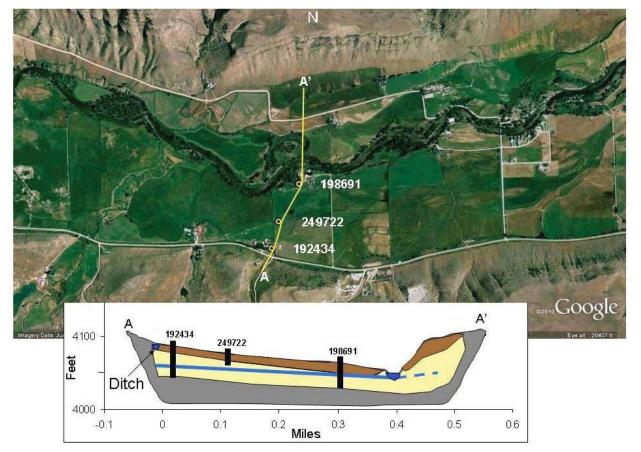
Figure 13. Cross section of the wells in the alluvial aquifer.
