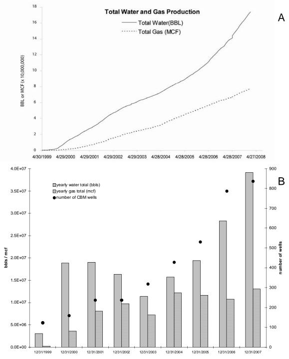
**Figure 19A**. Total water and gas produced since CBM production began in spring 1999 (data from MT BOGC on-line database). Water production climbs faster than gas production since early 2006 most likely due to more new CBM wells coming on-line.
