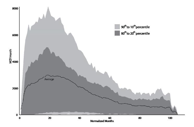
Figure 18. Normalized gas production in MCF per month for the Montana portion of the Power River Basin (data from MT BOGC web site). Solid line represents the average MCF produced, the light grey field represents the 10<sup>th</sup> to 90<sup>th</sup> percentile, the dark grey field represents the 20<sup>th</sup> to 80<sup>th</sup> percentile.
