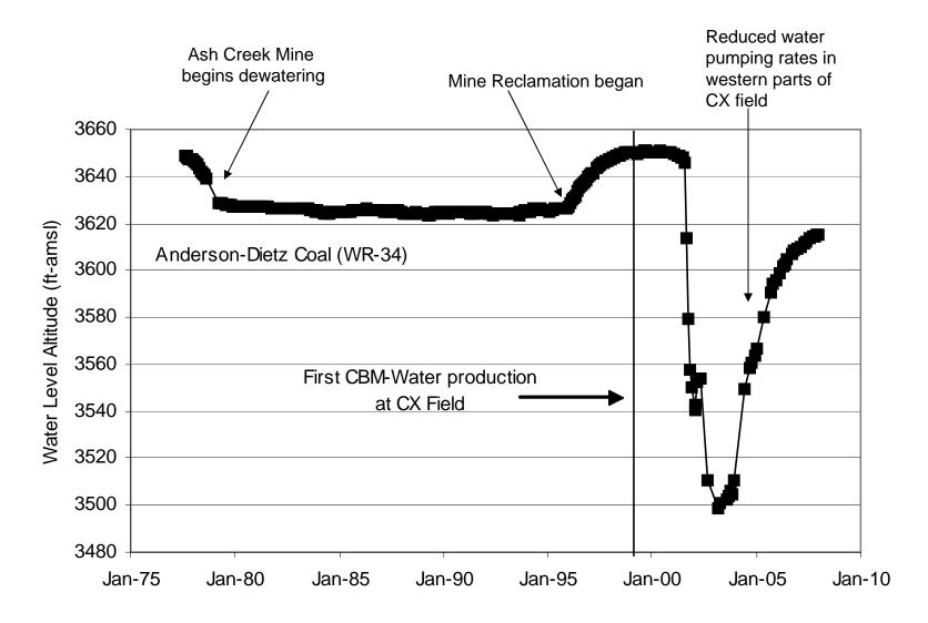
Figure 21. Water levels in the combined Anderson and Dietz coal (WR-34) in the Young Creek area respond to both coal mining and coalbed methane production. The water level recovered starting in 2003 in response to water production decreases in this portion of the CX field.
