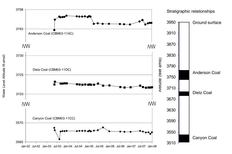
Figure 5 . A downward hydraulic gradient is evident between the Anderson, Dietz, and Canyon coalbeds at the CBM03-11 site.
