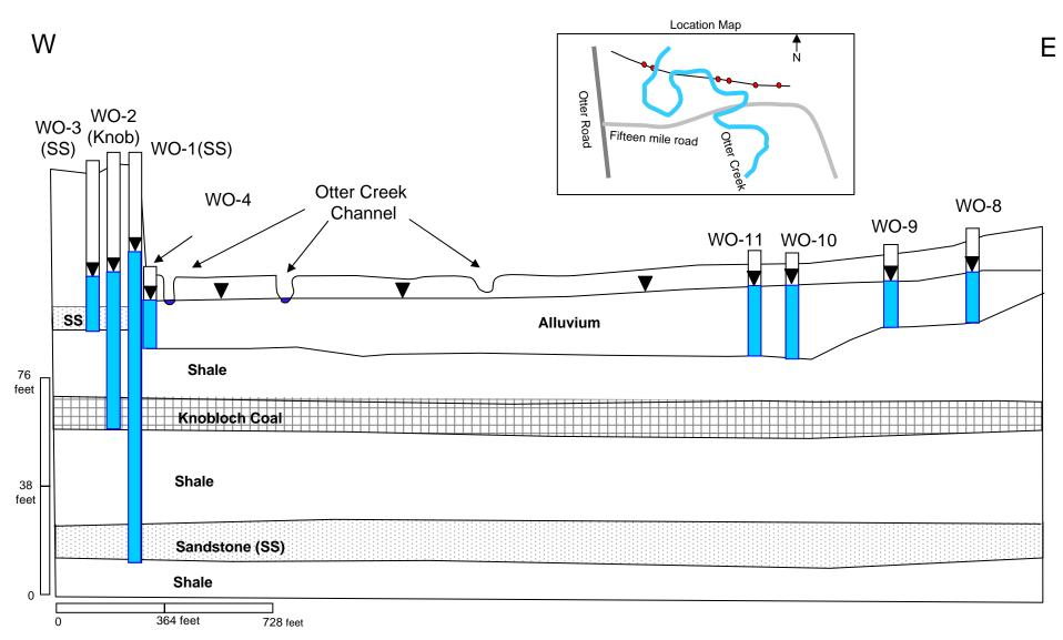
Figure 8. Geologic cross section for the Otter Creek alluvium and bedrock wells located in T05S R45E sec 23. Water levels in the alluvium are lower than the underlying bedrock aquifers. The water levels in the bedrock wells completed in stratigraphically deeper units are higher than those in shallower units. The water levels for this cross section were taken in February, 2007. Vertical exaggeration is 9.6:1.
