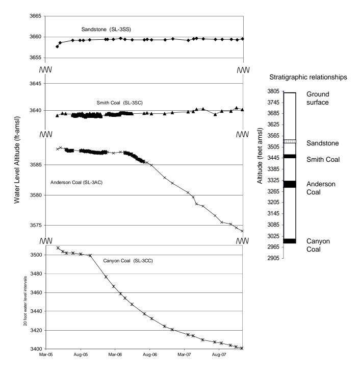
Figure 35. Water levels in the overburden sandstone and Smith coals are not responding to CBM development. However the water level in the Anderson and Canyon Coal have dropped about 13.5 and 103 feet respectively in response to CBM production.
