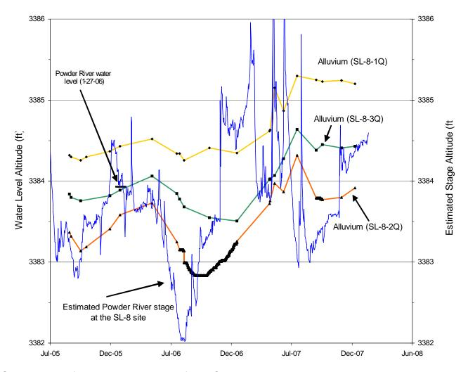
Figure 39. Ground-water flow in the alluvial aquifer at SL-8 is roughly parallel to the Powder River. The ground waterlevel trends follow river stage trends. The river alternates between gaining (summer) and loosing (winter). Estimated Powder River stage at SL-8 is based on stage at Moorhead gaging station (USGS data) and the surveyed river water-level altitude at SL-8 on 1/27/06.
