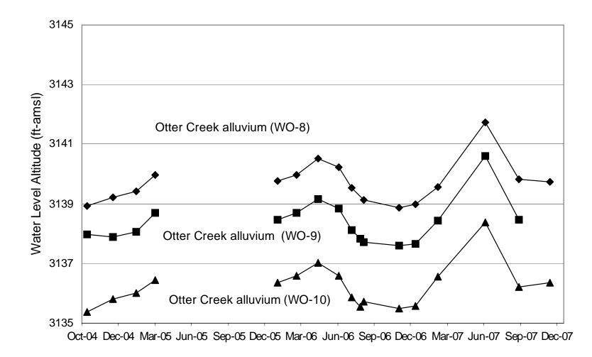
Figure 10. Water-level trends in the alluvium at the Otter Creek site probably relate to weather patterns. The alluvial aquifer appears to receive recharge from the bedrock aquifers in the area, based on the upward vertical gradient.
