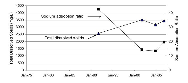
Figure 28. Water quality samples have been collected periodically from WR-17A. As the water level increased (see figure 26) the TDS also increased. At the same time the SAR is decreased due to the dissolution of calcium and magnesium salts.
