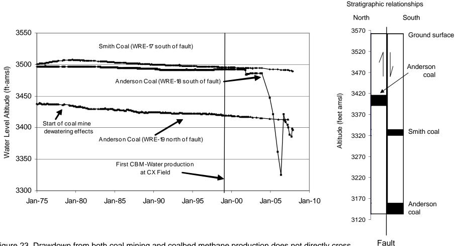
Figure 23. Drawdown from both coal mining and coalbed methane production does not directly cross faults in the project area. Mining has occurred north of this fault since the early 1970's and only minor drawdown has been measured at WRE-17 since the mid-1980's. The pressure reduction has probably migrated around the end of the fault. Coalbed methane production south of the fault is apparent in WRE-18 but not across the fault in WRE-19.
