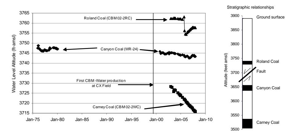
Figure 24. The long-term decrease in water levels in the Canyon Coal is probably related to precipitation patterns. The short period of record for the Carney coal at the CBM02-02 site does not indicate meteorological influence but has responded to CBM related drawdown since its installation. The Roland Coal has not been developed for CBM production and the water-level decline is not likely a response to CBM activities.
