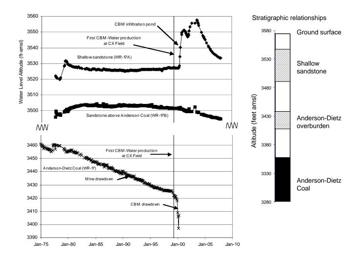
Figure 27. Long-term water-level trends in the Anderson overburden(WR-17A and WR-17B) in the Squirrel Creek area, may relate to precipitation patterns. These wells demonstrate the rise in water table in 1999 at WR-17A is believed to be in response to infiltration of water from a CBM holding pond. The water level in this aquifer is now dropping as the pond no longer receives water.
