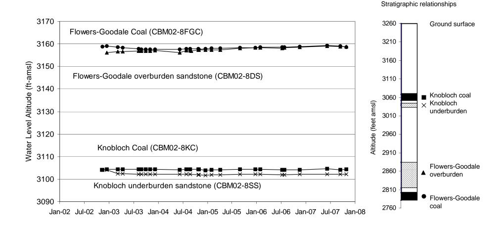
Figure 6. Water levels in wells completed in the stratigraphically deeper Flowers-Goodale units are higher than those in the shallower Knobloch coal units at the CBM02-08 site.
