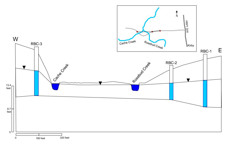
Figure 11. Cross section of the Rosebud creek site located in T06S R39E section 8. Water levels in this alluvial aquifer and surface water levels in Rosebud Creek are closely related. Well water levels are lowest in late summer and highest in early spring. The water levels at RBC-2 shows a correlation with the diurnal effect from the surrounding alfalfa plants. Water levels for this cross section were taken in January 2007.
