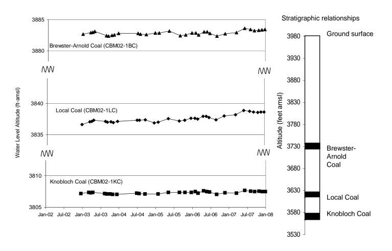
Figure 7. A downward hydrostatic gradient is evident between the Brewster-Arnold coal, local coal, and Knobloch coal at the CBM02-1 site.
