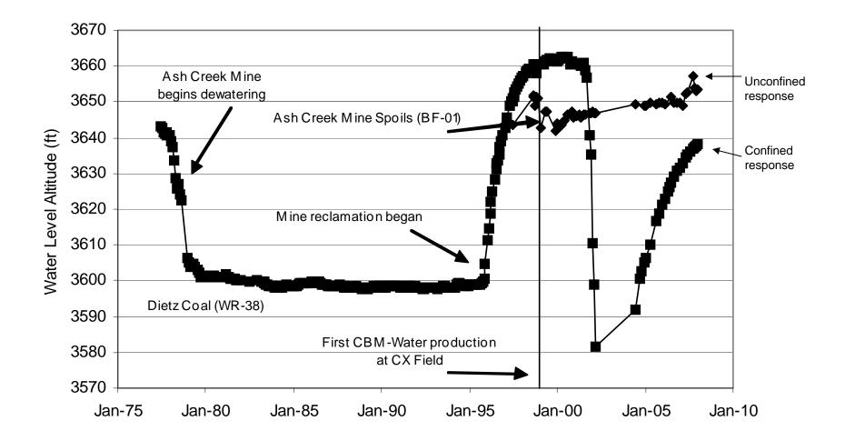
Figure 22. The mine spoils well is being dewatered for CBM production but the water levels show no response to the lowered water levels. However, water levels have decreased by 80 feet in the Dietz Coal in response to the CBM production.
