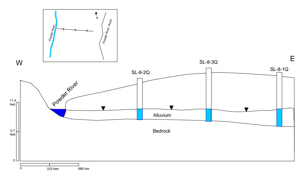
Figure 38. Cross section of alluvial wells south of Moorhead near the Powder River located in T09S R47E section 25. Ground water in the alluvium appear to flow parallel to the river. Water levels for this cross section were taken in January 2007. Vertical exaggeration is 58:1.
