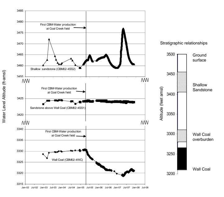
Figure 30. A downward hydraulic gradient is evident between the shallow sandstone, Wall overburden sandstone, and Wall coal at the CBM02-4 site. Water-level trends in the Wall coal and overburden are probably not related to meteorological patterns while those in the shallower sandstone may be. The water level in the Wall Coal aquifer has decreased 11ft in response to CBM development. No CBM effects are seen in the shallower aquifers.
