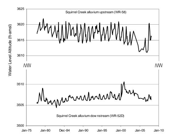
Figure 29. In addition to normal annual cycles, long-term precipitation trends affect water-table levels in the Squirrel Creek alluvium. Upstream of CBM production Squirrel Creek alluvium is not influenced by CBM production (WR-58), but adjacent to CBM production the water level rise since 1999 and fall during 2004 likely relates to infiltration ponds located in between these sites (WR-52D).
