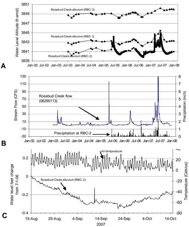
Figure 12. A) Ground-water levels are typically higher during wetter times of the year at the Rosebud Creek alluvium site. B) Rosebud Creek stream flow follows precipitation trends. C) Diurnal drawdown occurs in the aquifer due to the surrounding alfalfa fields as shown by the correlation between water levels and air temperature. Note that the X axis on C is reduced to a shorter time scale.
