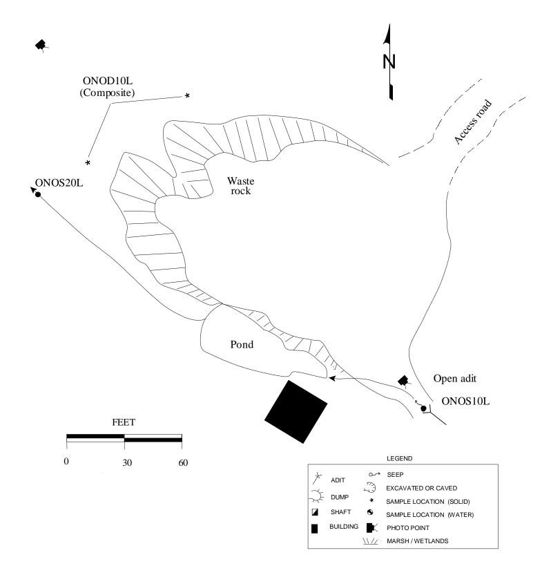
Figure 4. The North Ontario mine adit was open and discharging water to a small pond (8/9/95). The road to the site is not well marked but showed recent traffic.
