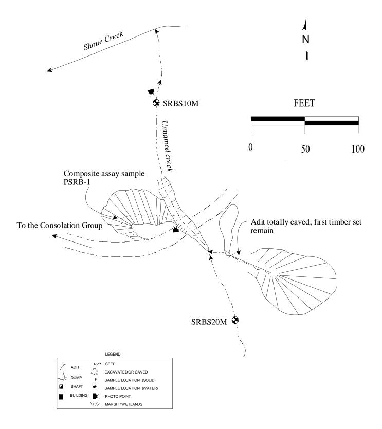
Figure 22. Rex Beach's discharge joins with the flow in an unnamed creek, as mapped 10/12/94.
