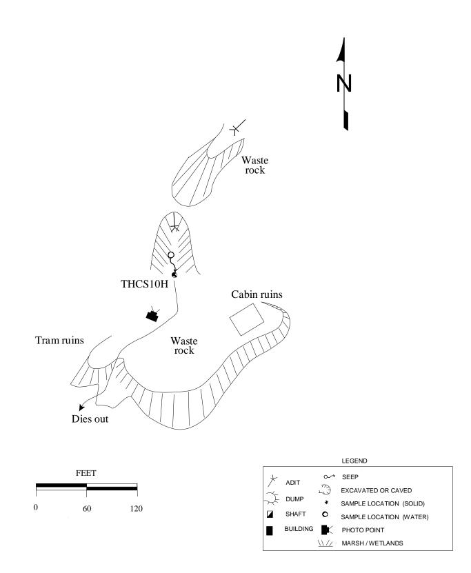
Figure 8. The Hub Camp mine (8/3/95) consisted of two caved adits; the lower adit was discharging a small amount of water. The stream infiltrated the ground within a short distance from the base of the dump.
