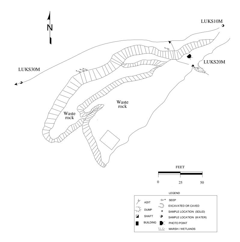
Figure 18. The upper Kimball mine is below the Big Dick mill, the Treasure Mountain mine, and several other mines and mills. The adit was caved and was discharging water to an unnamed tributary of the Little Blackfoot River (9/28/95).
