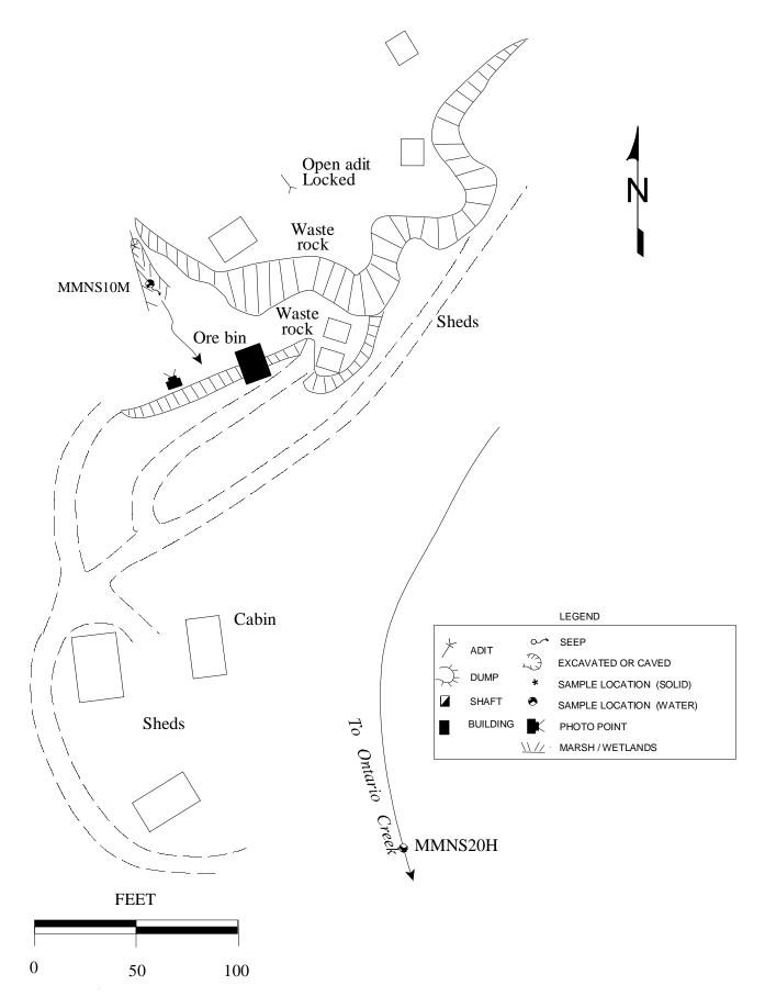
Figure 13. The Monarch mine was apparently active (9/27/95); the upper adit had recently been repaired. The lower adit was discharging about 0.3 gpm.
