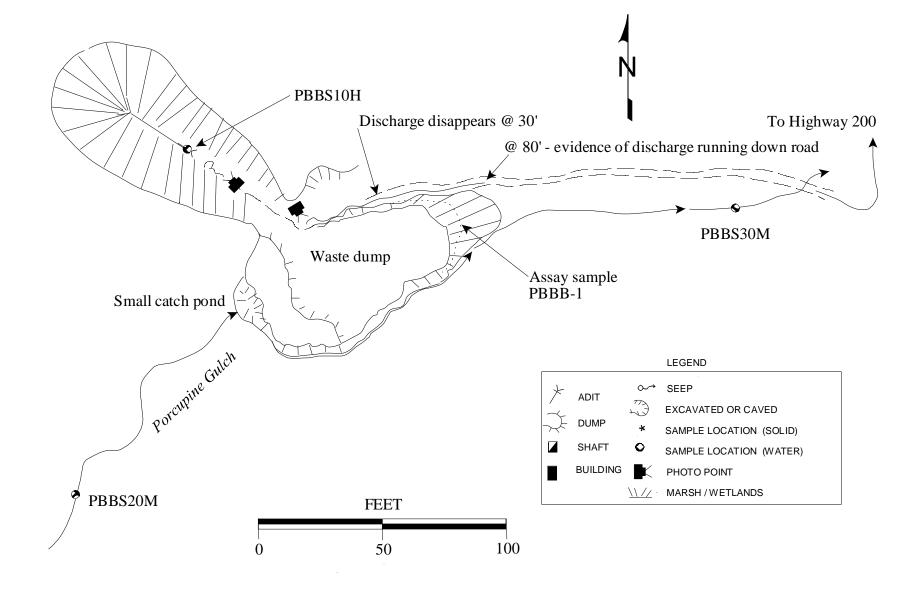
Figure 24. Bobby Boy mine on Porcupine Gulch discharges less than one gpm as mapped 09/08/94.
