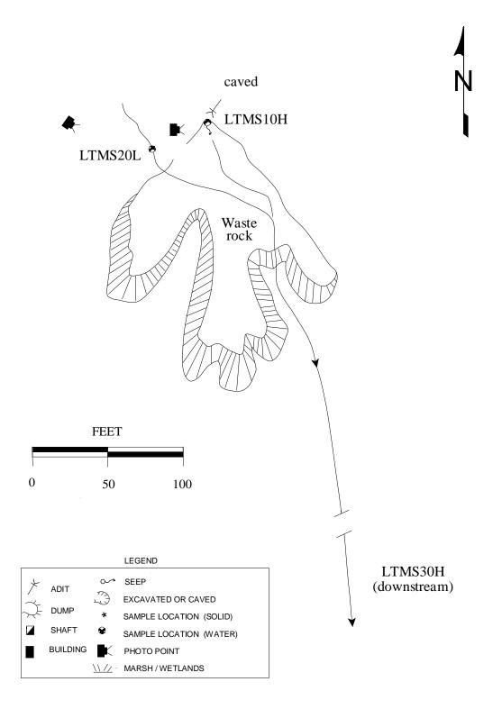
Figure 16. The Treasure Mountain mine adit was discharging about 6 gpm. There was evidence that the adit has greater flows at other times of the year. The lower waste-rock dump is not shown.
