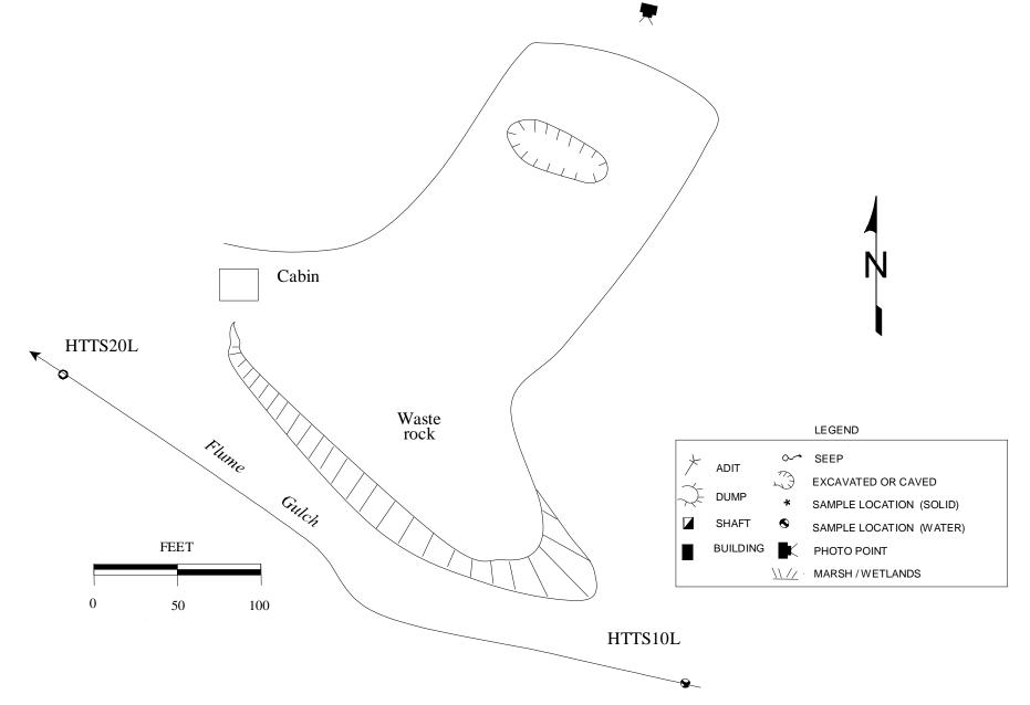
Figure 11. The Third Term mine had been reclaimed at the time of the visit (9/26/95). On an earlier visit by the geologist, water was seeping from the collapsed adit.
