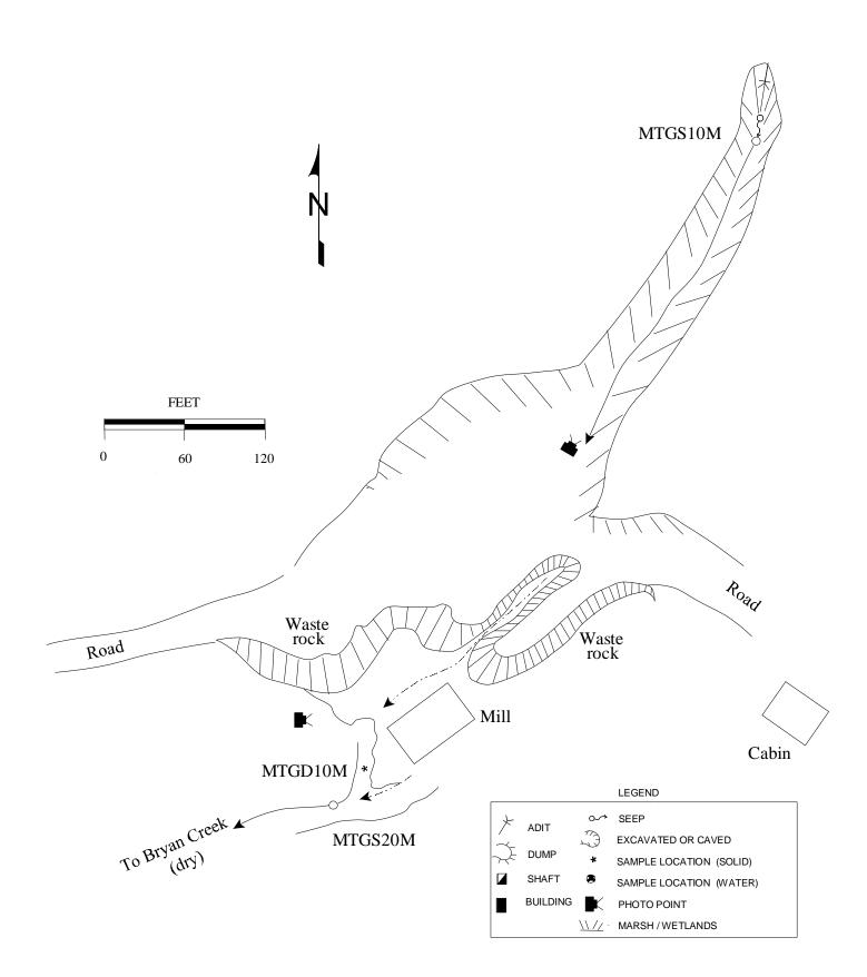
Figure 3. The Telegraph Creek mine (8/3/95) was discharging water from the adit and from springs below the mill. The site is bisected by the main road between Telegraph Creek and Tenmile Creek.
