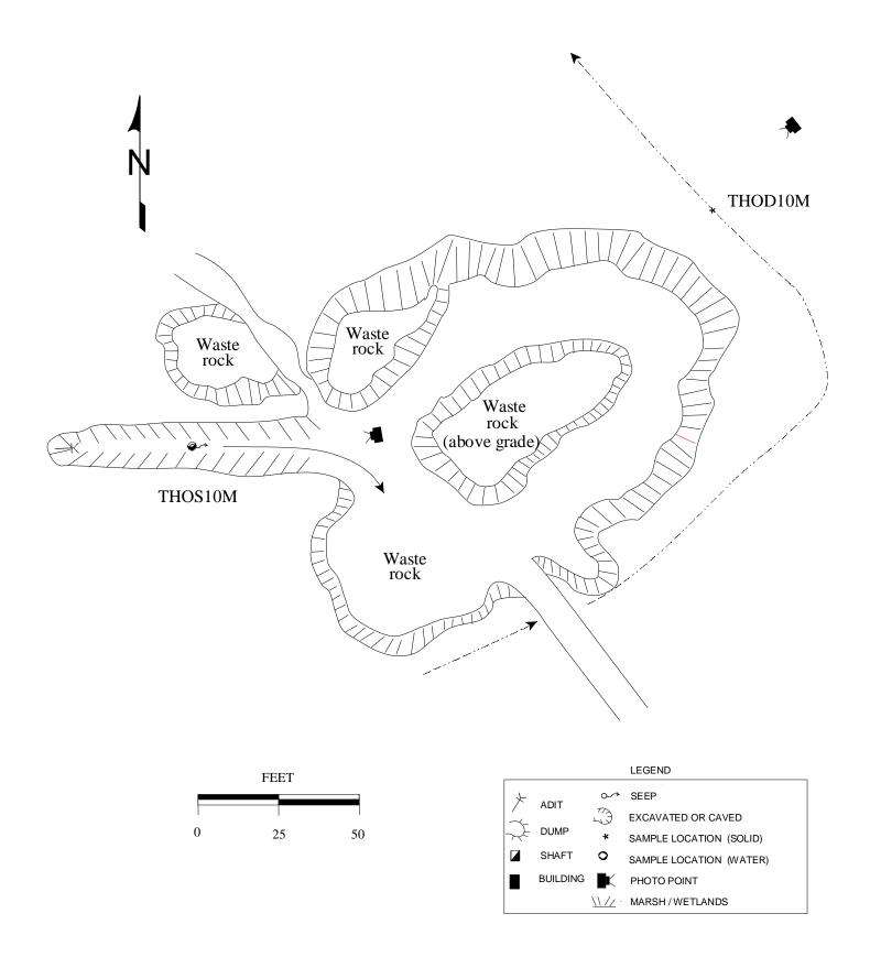
Figure 7. The Hope mine (8/9/95) was discharging water from a caved adit. There were several dry stream beds that probably flow during snowmelt and large storms.
