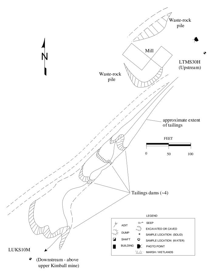
Figure 17. The Big Dick mill tailings extended about 500 feet downstream of the mill (9/28/95). The lateral extent was difficult to distinguish in some areas.
