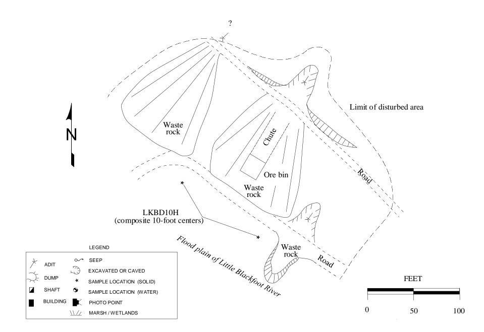
Figure 15. The Kimball mine had no site discharges at the time of the visit (10/6/95); however, waste material had been eroded and deposited in the flood plain of the Little Blackfoot River.
