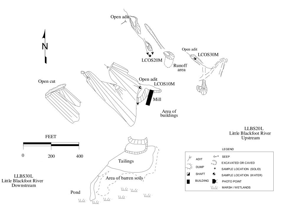
Figure 19. The Charter Oak mine and mill covered a large area next to the Little Blackfoot River (10/6/95). The tailings are in the flood plain of the river.
