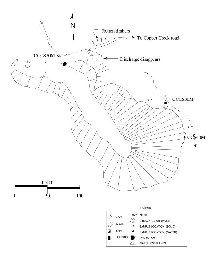
Figure 28. Several springs and an adit discharge emerge from the lower workings of the Copper Camp site, 08/22/94.
