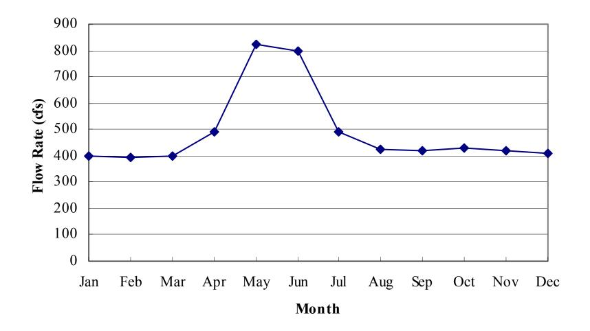
**Figure 4.2** Average monthly flow, Madison River near West Yellowstone, Montana (U.S. Geological Survey Station No. 06037500). Period of record: 1913 to 1995. Data source: Shields *et al.* (1996).
