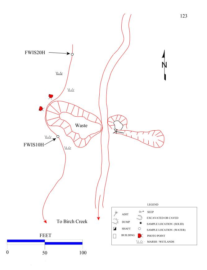
**Figure 3.31** A small waste dump lies in the Farlin Gulch drainage and is actively being eroded, as mapped July 16, 1996.
