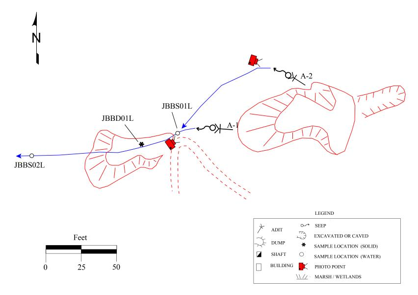
Figure 4.4 Site map of the Branham Basin mine, September 1996. The adit discharges join and flow into a marshy area.
