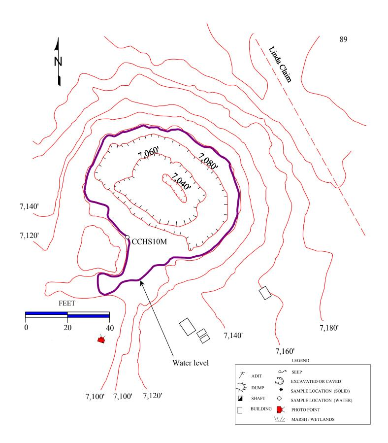
**Figure 3.10** The Calvert pit showing water level as mapped October 31, 1961 by Anaconda Company geologists. Water sample location CCHS10M from the MBMG study is shown also.
