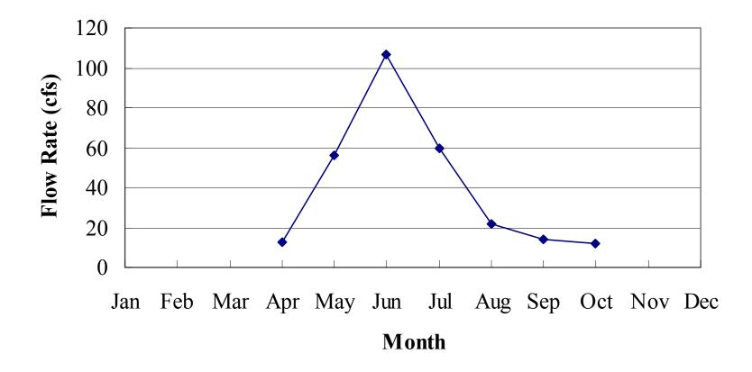
**Figure 2.1** Average monthly flow, Odell Creek above Taft Ranch, near Lakeview, Montana (U.S. Geological Survey Station No. 06008000). Period of record: 1993 to 1995. Data source: Shields *et al.* (1996).
