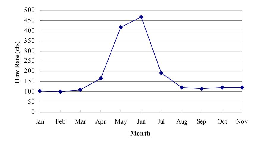
**Figure 4.1** Average monthly flow, Ruby River above the Ruby Reservoir. (U.S. Geological Survey Station No. 06019500). Period of record: 1938 to 1995. Data source: Shields *et al.* (1996).
