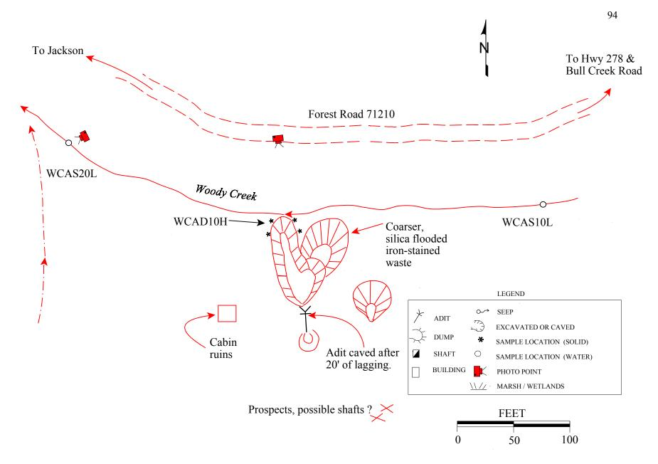
**Figure 3.13** The small waste dump at the Carney mine contacted Woody Creek during times of high water but was not in contact on August 11, 1997.
