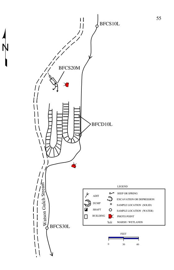
**Figure 2.16** At the Watson Gulch mine, there is a small adit discharge and a streamside wasterock dump (10/8/96).
