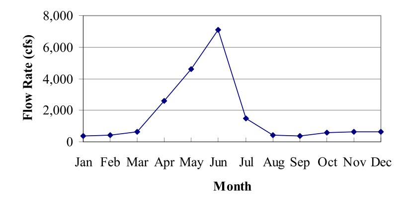
**Figure 3.1** Average monthly flow, Big Hole River near Melrose, Montana (U.S. Geological Survey Station No. 06025500). Period of record: 1924 to 1995. Data source: Shields *et al.* (1996).
