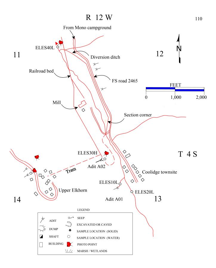
**Figure 3.23** Schematic of the Elkhorn mine and mill on Elkhorn Creek taken from the Elkhorn Hot Springs 7.5-min. topographic map. The Upper Camp Elkhorn mine also is shown.
