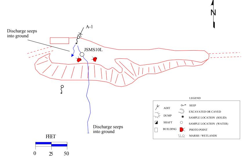
**Figure 4.44** Site map for the Smuggler mine, September 1996. The adit discharge sinks into the ground about 200 to 300 feet from Mill Creek.
