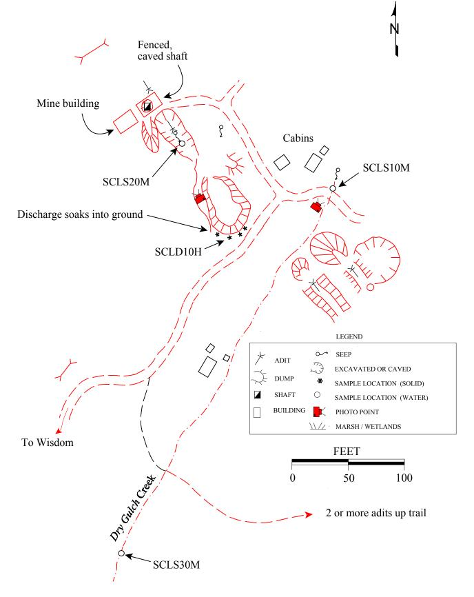
**Figure 3.16** Seeps from the adit at the Clara and the surrounding hillside form Dry Gulch Creek, a small tributary to Steel Creek (August 1997).
