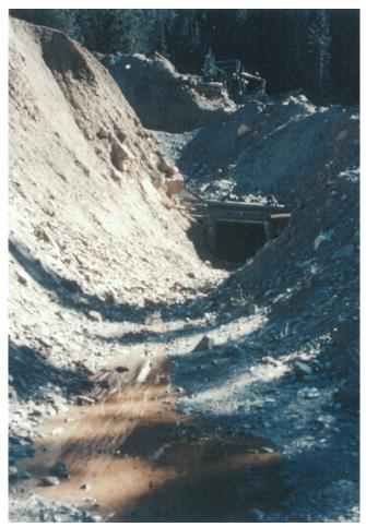
**Figure 4.48** The lowermost adit at the Uncle Sam mine is open and has an iron-stained discharge.
