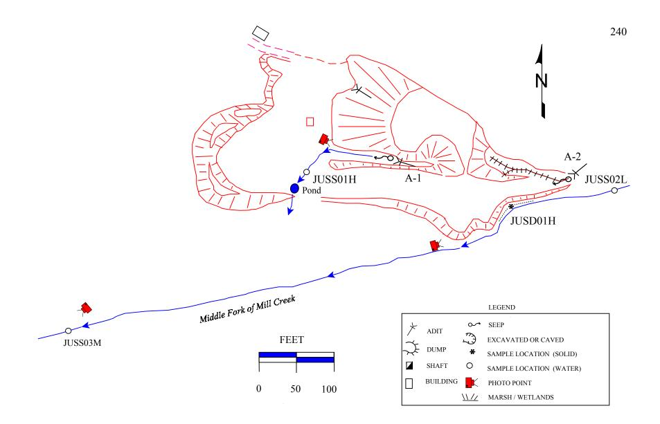
Figure 4.47 Site map of the Uncle Sam mine, September 1996. Waste rock is in contact with the Middle Fork of Mill Creek.
