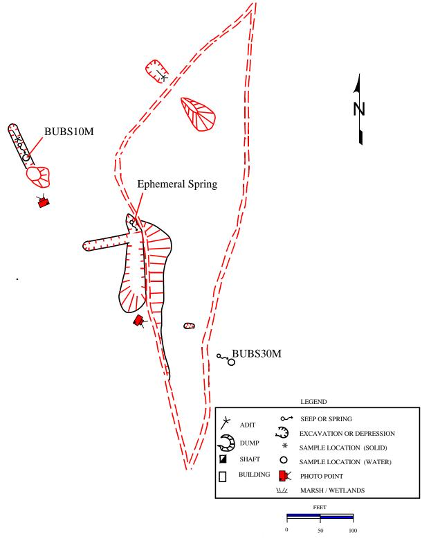
**Figure 2.13** A small iron-oxyhydroxide stained spring flows from the upper adit at the Pay Day group, as mapped in September 1996.
