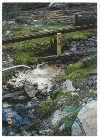
**Figure 3.38** The Ibex mine had an adit discharge that flowed at 5 gpm; no signs of AMD were evident.
