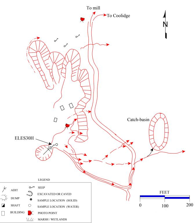
**Figure 3.22** The Elkhorn mine discharges onto the waste dump and has seeps at the south end of the same dumps, as mapped September 10, 1996.
