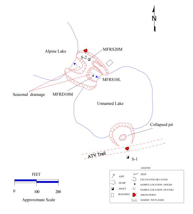
**Figure 4.9** Site map of the Frisbee mine showing waste rock in contact with the lakes and the location of shafts, September 1996.
