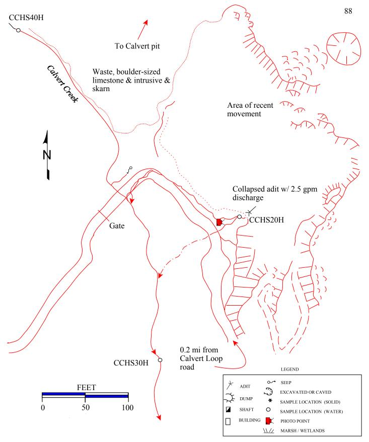
**Figure 3.9** Site map of the Calvert mine area, August 1996. Slumping has occurred on the slope above the adit.
