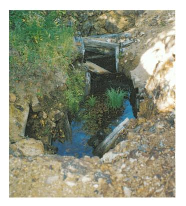
Figure 3.50 A shaft at the Park mine is flooded and has a small discharge at the north end.
