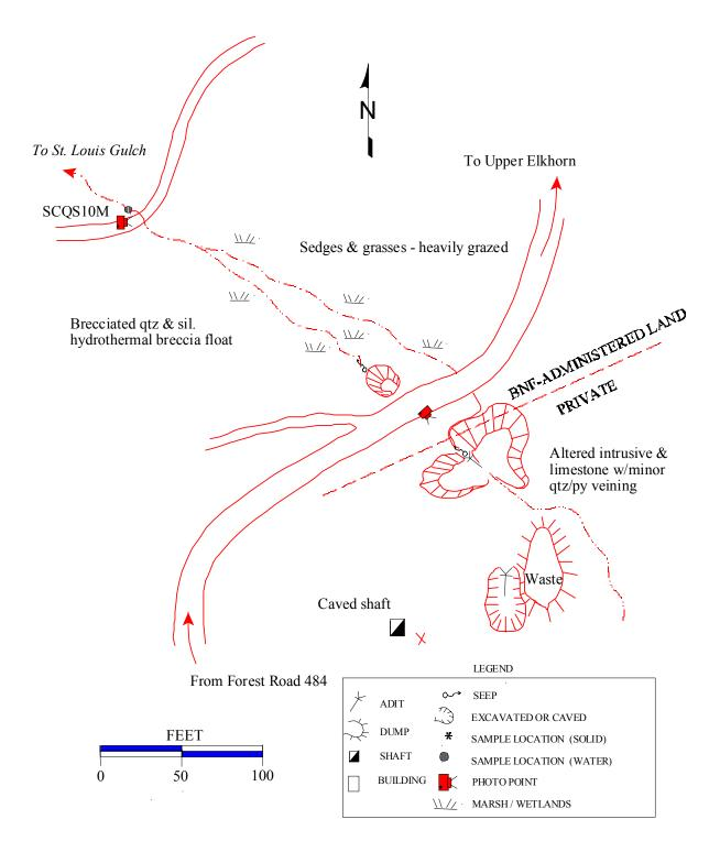
Figure 2.7 The Copper Queen patented claim had a small discharge that flowed through a culvert and down toward St. Louis Gulch, as mapped September 11, 1996.
