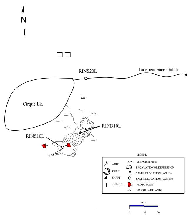
**Figure 4.12** At the Independence Gulch Claim No. 1, an adit discharge flows into a marsh adjacent to a small cirque lake (8/27/96).
